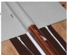
In thinking about this design, I wondered if the aluminum on top of the tube was decreasing the efficiency of the heat transfer process by introducing a layer of material between the sun and the tube to which you are trying to transfer the heat.
