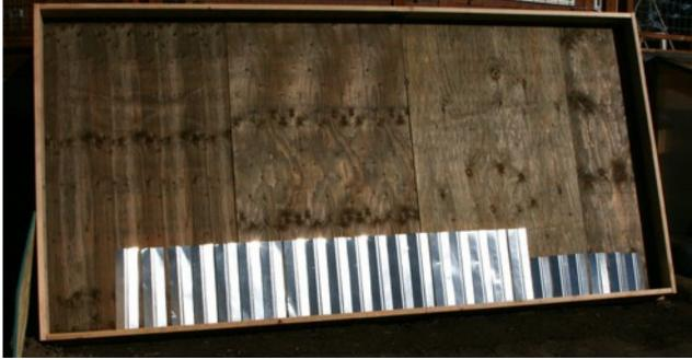
In this pic, I am placing the absorber fins in the frame for painting.
