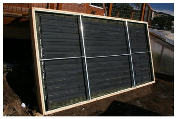
Here is the finished collector with glazing and sheet metal covering the perimeter:
