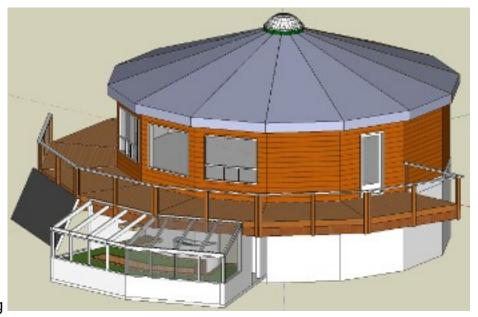
the day and release it overnight. The hydronic system will add supplemental heat to the GH when needed and will also provide domestic hot water (DHW) heat to the house. You can see the planned solar collector to the left of the GH. In addition to providing thermal mass, the pond might ultimately be used to provide a waterfall feature to provide evaporative cooling in the summer. A bonus will be to add fish and water plants for fun.
